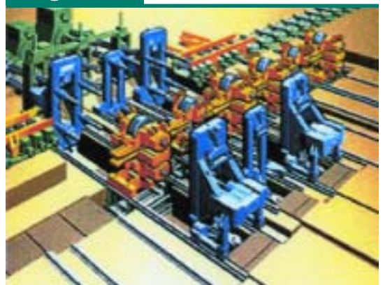
A complete roll change of all three stands, including guides, is accomplished in less than 25 minutes using the compact cartridge stand changing procedure.
